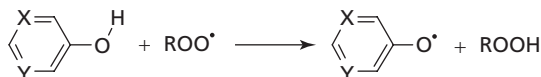
Figure 3 Reaction of peroxy radicals with phenol ( X = Y = \text{CH} ), pyridinols ( X = \text{N} ; Y = \text{CH} ) and pyrimidinols ( X = Y = \text{N} )
